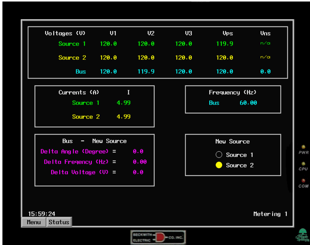
Figure 8 MBTS Metering Screen
